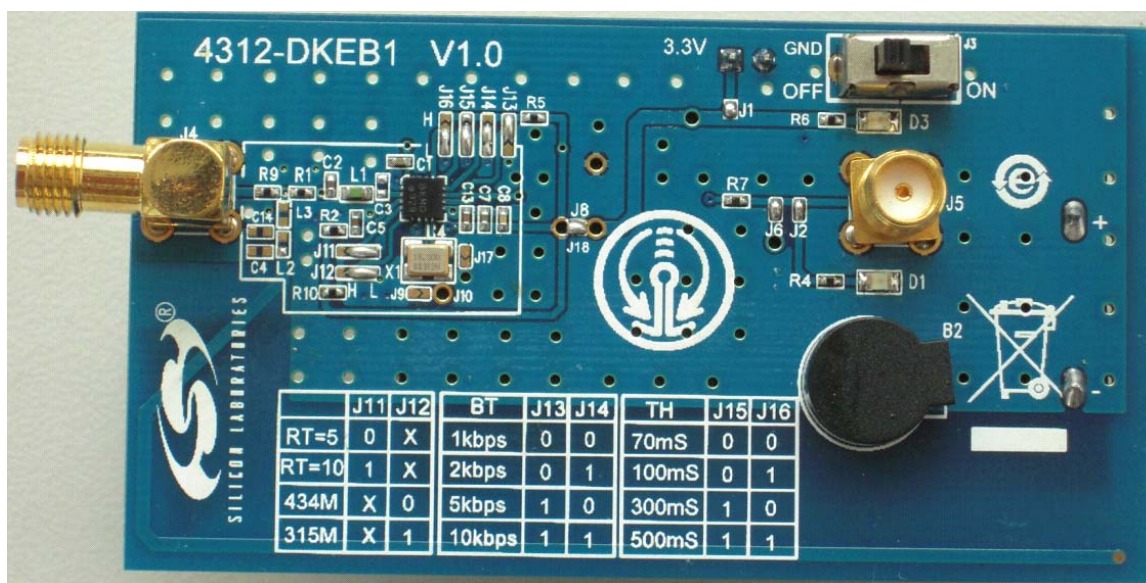
Figure 1. Si4312 DEMO Board Top Side
