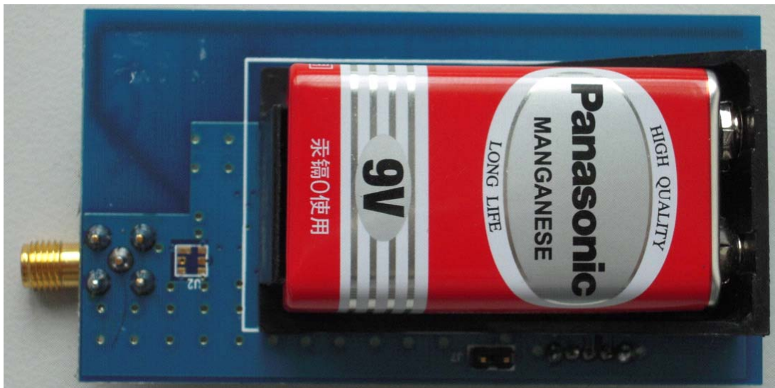
Figure 2. Si4312 DEMO Board Bottom Side with 9 V Battery
